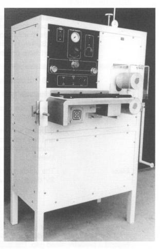
The gap setting between the rollers is adjusted either by fixed height interchangeable spacer blocks or through the use of the optional gap adjustment option. A storage shelf for height blocks is provided in the access door. An electric heater mounted under the tape feed table pre-heats the Honeycomb as the tape is applied.
